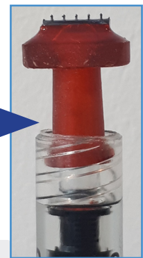
Fig. 4 Microneedle array attached to industry-standard Leur Lock on a syringe
