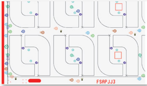
Tooling hole placement
