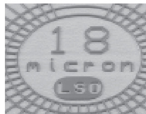
Fine lines/spaces of 18µm
