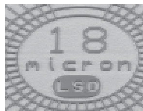
Fine lines / spaces of 18µm
