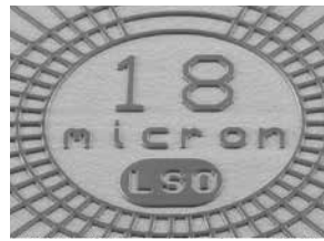
Fine lines and spaces of 18µm for the most advanced applications
