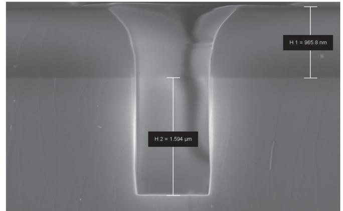
Fig. 4 Power trench (1.6μm deep) with no micro-trenching, etched at 0.75μm/min
