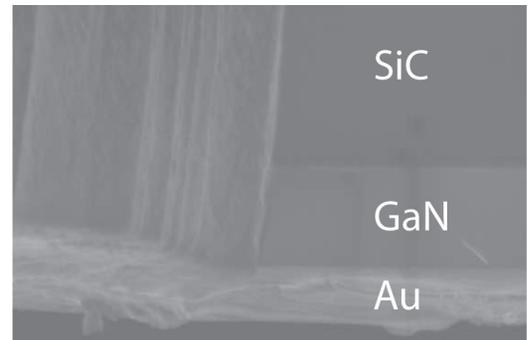
Fig. 2 GaN etch to underlying Au layer
