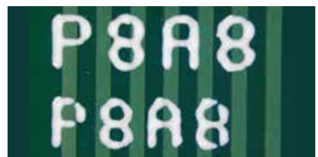
PREVIOUS: 0.7 & 0.6 mm text before DotStream Pro Technology™ One pass, 26 sec*.
