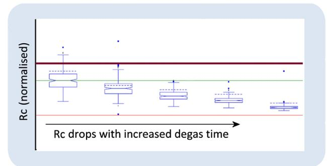
Fig 2 Benefit of increasing degas time - Reduced Rc
