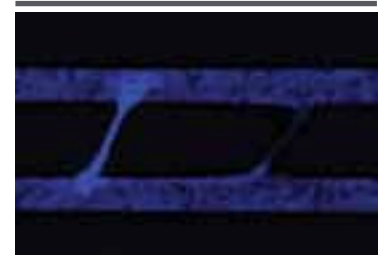
Blue light image - clear distinction between dust and fine short (dust is much brighter)
